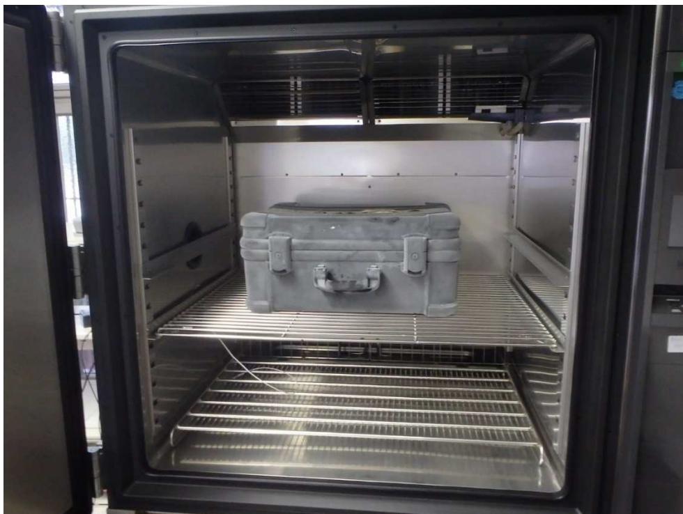
Illustration 5: Frozen Container in hot chamber
