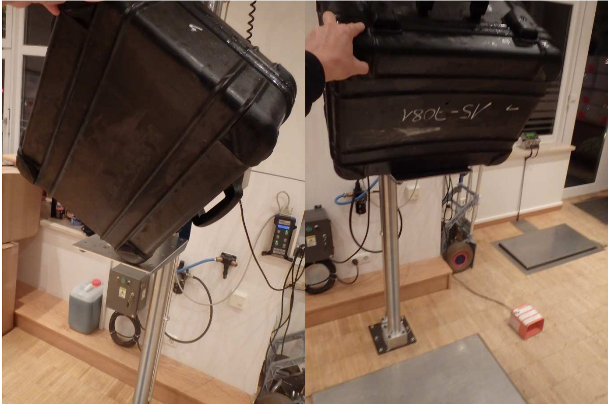
Illustration 8: Setup drop table (corner and edge drop)
