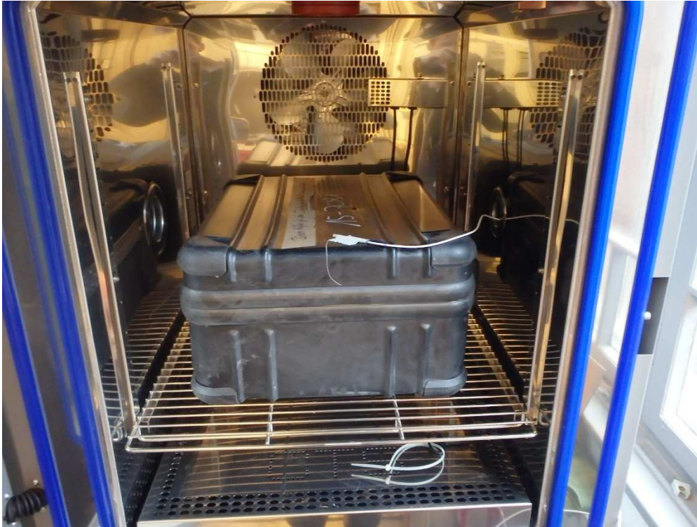
Illustration 3: Test setup cold
