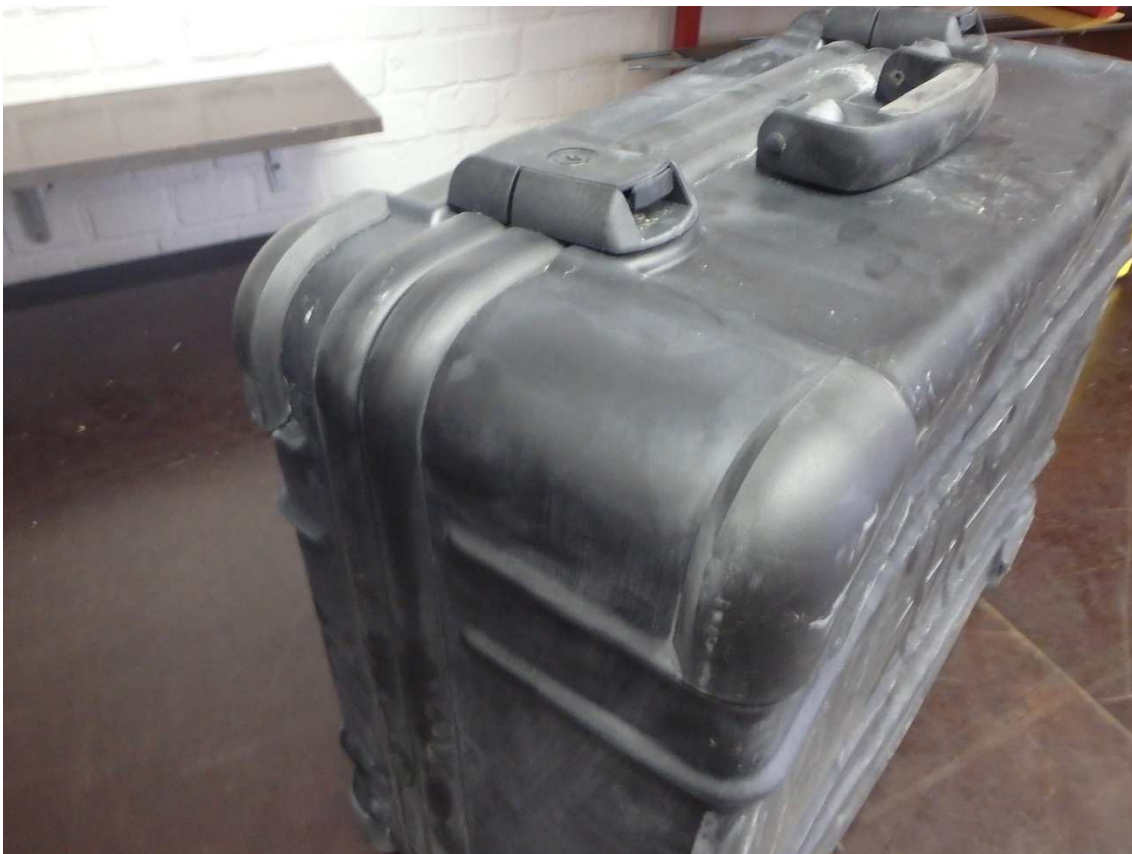
Illustration 7: Container corner during temperature shock test
