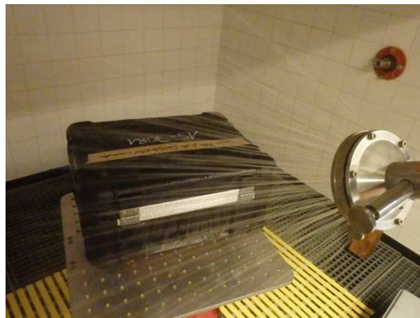
Illustration 7: Test Proceeding IP X4
