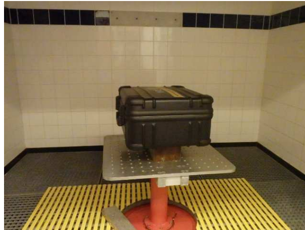
Illustration 6: Test Setup Wet-Chamber
