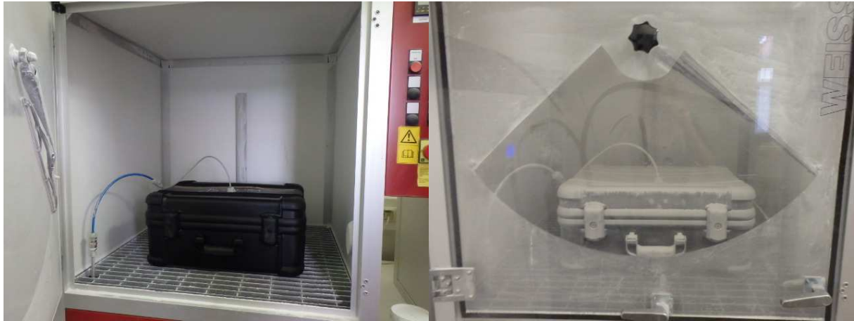
Illustration 4: Test Setup Dust Chamber; Specimen after Test
