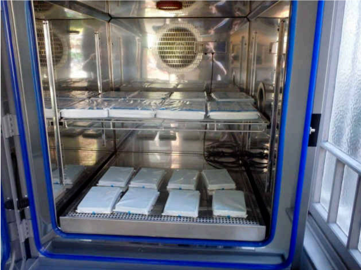
Figure 3: Pre-Conditioning – Setup Cooling Pads
